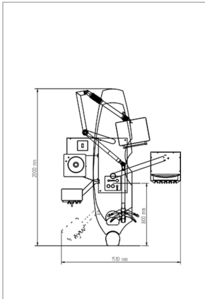
Dimension sheet for the **L1-S600**, **L1-ECO** and **L1-ECO-AIR** models with an assistant's device.
