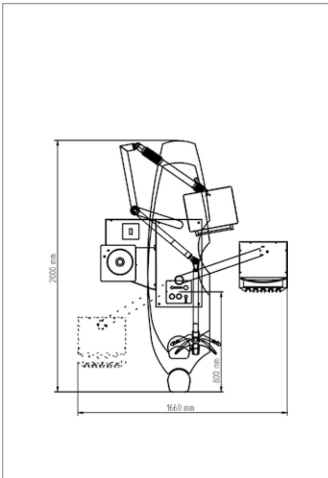
Dimension sheet for the **L1-ECO AIR**, **L1-ECO** and **L1-S300** models. The doctor's device with integrated suction tubes can be swivelled to the doctor's or the assistant's side.
