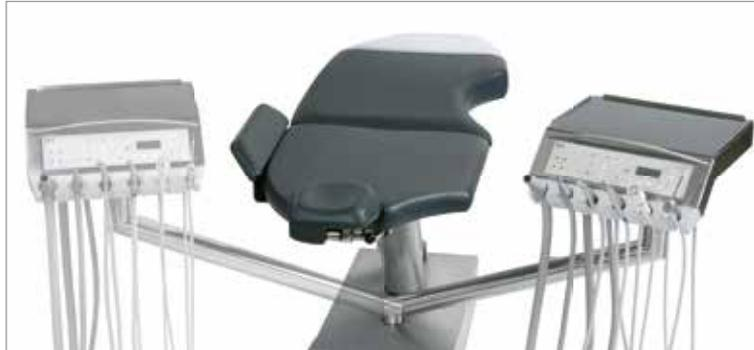
The basic equipment of the doctor's device includes the small and large suction tubes. The doctor's device can be equipped with up to four instruments, a brushless 100-40,000 rpm LED-micromotor, a turbine connection, a Piezo scaler and a function syringe. The EM-12 L electric motor is small but mighty. It is suitable for restoration and prosthetics as well as for endodontics and prophylaxis. The extremely small electric motor is the perfect synergy of ergonomics and performance.
