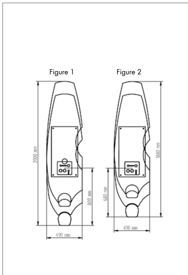
This dimension sheet shows the **L1-SOLO** model with a long back rest (figure 1) and the **L1-SOLO** model with a short back rest (figure 2).
