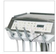
The doctor's device can be equipped with 6 instruments, brushless 100-40,000 rpm LED micromotors, a turbine connection, a Piezo scaler and a function syringe. The EM-12 L electric motor is small but mighty. It is suitable for restoration and prosthetics as well as for endodontics and prophylaxis. The extremely small electric motor is the perfect synergy of ergonomics and performance.
